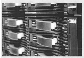
Figure 2-36 An array of hard disks in a server, arranged to provide data redundancy.
