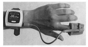
Figure 12-4 A monitoring device which measures blood oxygen levels and pulse rate.
