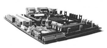
Figure 2-27 A typical computer motherboard
