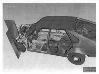
Figure 2-2 Supercomputers can be used to run computer models of car crashes, simulating physical forces and damage.
