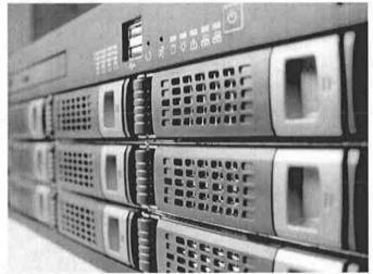
Figure 4-1 Many modern servers are blade servers, making it easy to connect many of them into a server enclosure (above).
