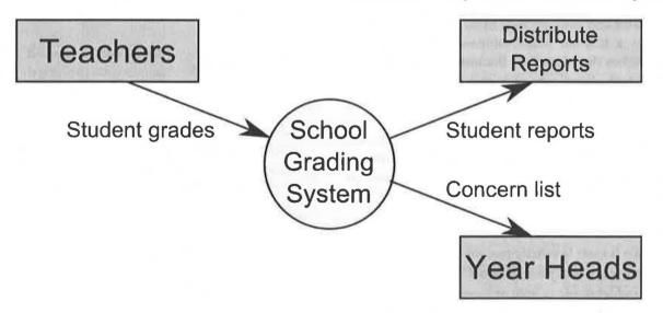
**Figure 15-6** A system context diagram which shows the relationship between the IT system (a school grading system) and external sinks. *Teachers* and *Year Heads* are clearly external stakeholders who send and receive data. Although *Distribute Reports* is a process, it is a physical task which is outside the boundary of the IT system (this would be determined by the requirements specification).
