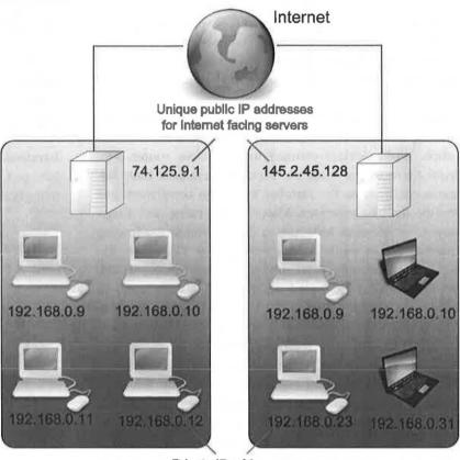
Private IP addresses used inside the LAN Figure 4-12 Private IP addresses are used on a LAN
