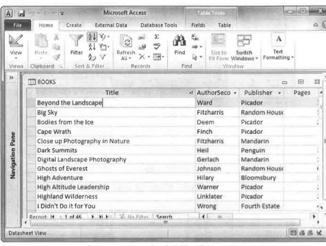
Figure 3-7 Database software structures data in tables, fields, and records
