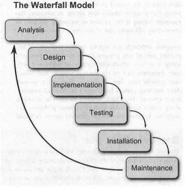
Figure 15-14 The traditional Waterfall model of software development, in which each stage is completed before moving onto the next.
