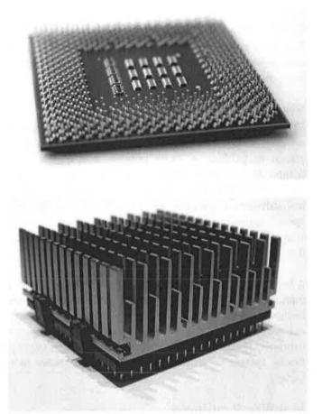
**Figure 2-26** The underside of a microprocessor (top). The gold pins are used to provide a connection with the motherboard. The top side of the processor with a heat sink attached (bottom). The heat sink's fins increase the surface area to aid cooling.
