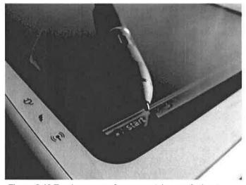
**Figure 2-13** Touch screens often use a stylus pen for input, and are common on mobile devices where there is no space for a regular sized keyboard.
