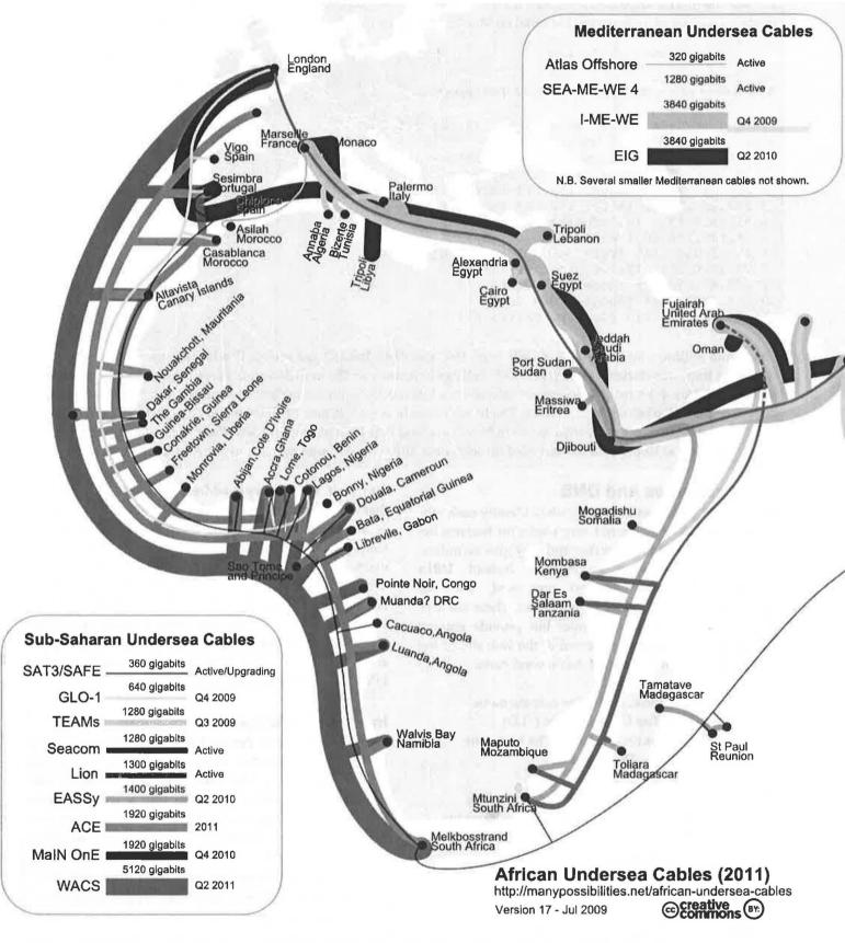
Figure 4-14 Undersea cables form the majority of the African Internet backbone. Connectivity is carried into the African interior through land based backbones which connect with the undersea cables.
