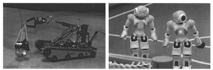
Figure 16-11 A US Navy bomb disposal robot (left); Robots designed to play football in the RoboCup league (right)
