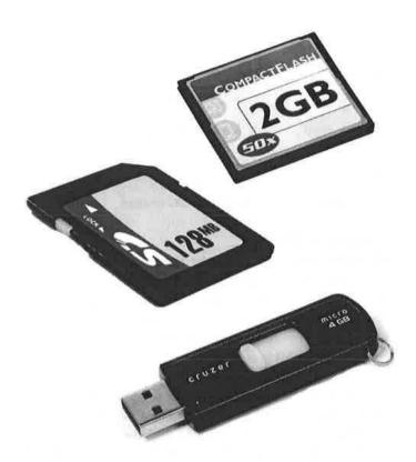
Figure 2-33 Various solid state memory: CompactFlash (top), SD (middle), and a USB flash drive (bottom).
