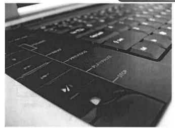
Figure 2-9 Multimedia buttons allow quick access to additional functions
