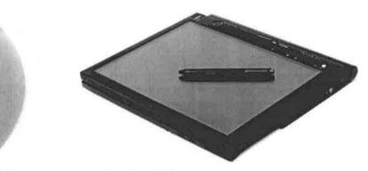
Figure 2-12 Two common input methods-a trackball (left) and touch screen with stylus (right)
