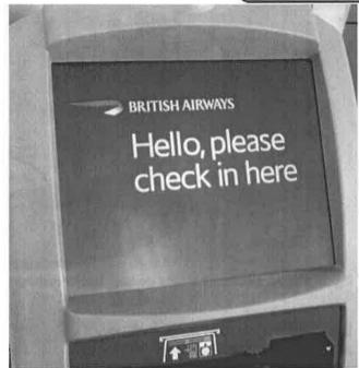
**Figure 2-14** Self-service check in machine at London's Heathrow airport. Using a touch screen and a software keyboard, machines like this can easily switch between several different languages and provide accessibility options.
