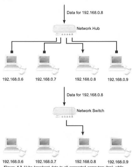
Figure 4-3 Hubs broadcast data to all connected computers (top), while switches send it only to the intended recipient (bottom)
