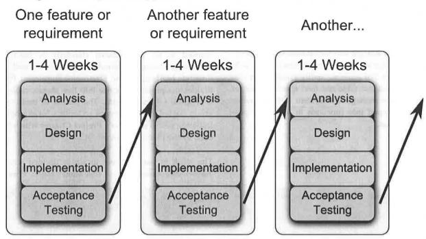
Figure 15-15 The agile model of software development breaks development down into shorter time periods
