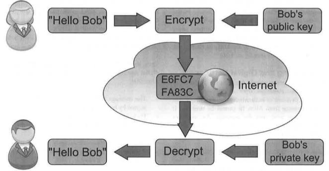
Figure 5-19 Public key encryption uses a key pair to remove the need of communicating a secret key over a network.
