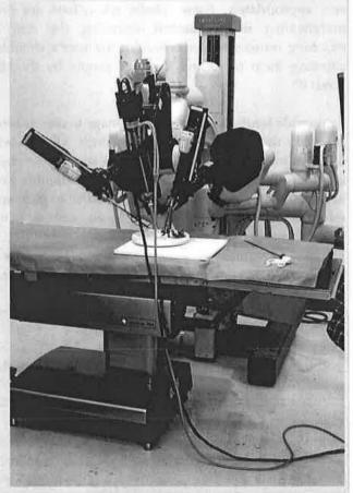
Figure 12-8 Patient-side part of the Da Vinci surgical system. The surgeon operates the robotic arms from a separate console (not shown).
