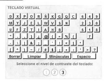
**Figure 2-10** A virtual keyboard used by an online banking site. The positions of the keys are randomized to prevent spyware from capturing passwords.
