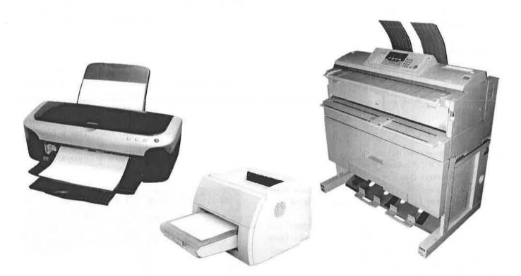
Figure 2-23 Printers come in many forms: inkjet printers (left) are often used with desktop computers as they offer good value for money; laser printers (middle) offer faster print speed and higher quality; specialised art printers (right) are used for larger print sizes and professional quality.
