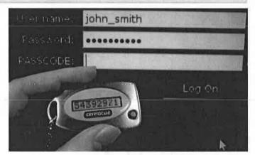
**Figure 5-1** A security token displaying a one time passcode, used in addition to a username and password for authentication.
