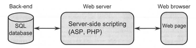
Figure 9-24 Data drive web sites use server side scripting tools to access a database and produce web pages using the results
