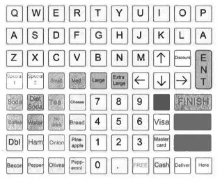
Figure 2-11 A concept keyboard that might be used in a restaurant to speed up the entry of orders
