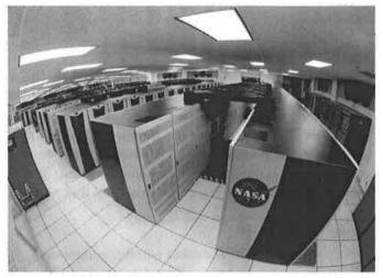
**Figure 2-4** The NASA Columbia supercomputer, used for advanced computer modelling and simulation. Columbia has 10240 processor nodes, 20 TB of primary storage, 440 TB of secondary storage, and can perform over 51 trillion operations per second. Columbia runs Linux and custom software to perform advanced mathematical modelling and simulation of space for future NASA missions<sup>4</sup>.
