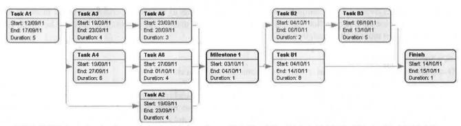
Figure 15-5 A PERT chart showing the project schedule from figure 15-3. The Critical Path is highlighted (Tasks A1, A4, A6, Milestone 1, B1, Finish)
