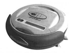
Figure 16-15 Small domestic robot for cleaning floors
