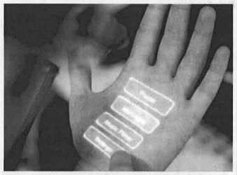
Figure 2-21 A user selects from menu options projected onto their hand using the Skin Input system. (Image courtesy of Microsoft Research and Carnegie Mellon University)
