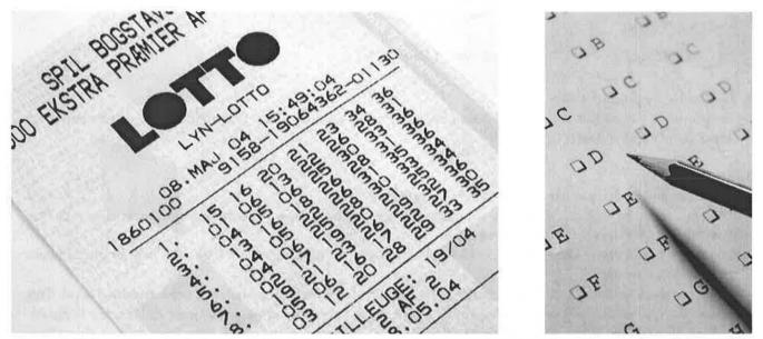
**Figure 2-18** Scanning technologies: Optical Mark Recognition recognises pen and pencil marks as they are placed in the boxes—the numbers are there for the human to read—the computer determines the answer by the position of the box on the page.
