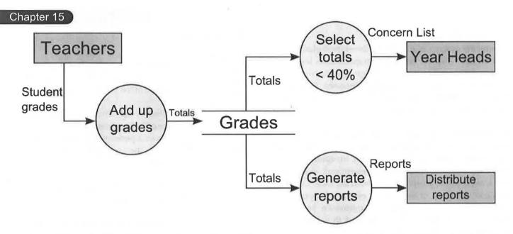
Figure 15-8 A Data Flow Diagram showing the school grading system depicted in figure 15-7. Although there is more detail than a system context diagram, each process represented could still be further broken down.
