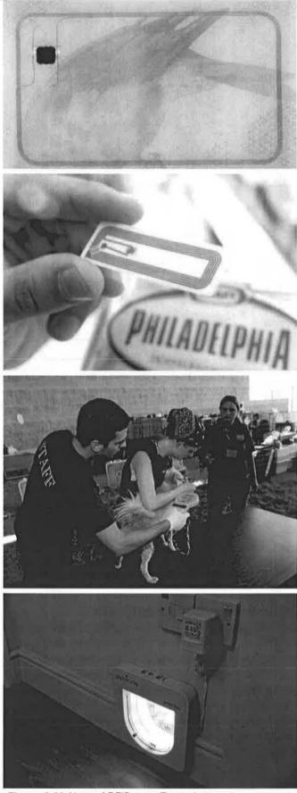
**Figure 2-20** Uses of RFID tags. Top to bottom: in a passport; in groceries; embedded in animals to aid identification; in a car flap which opens only for a specific animal, using a tag in its collar.
