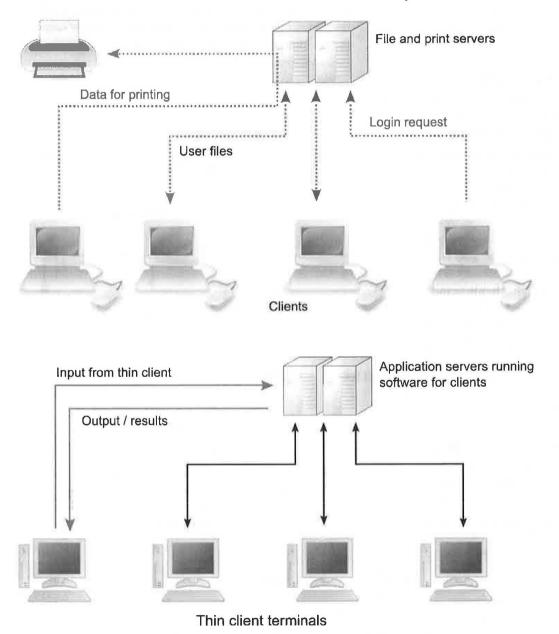
Figure 4-4 In client / server networks (top), servers centrally manage access control and provide a single location for file storage. In thin client networks (bottom), servers provide even more functionality, even running applications on behalf of the clients, which merely provide the input and output.
