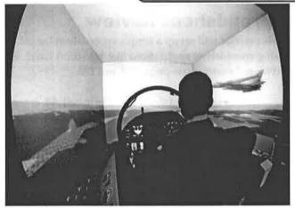
Figure 8-13 Simulators often use multiple screens to 'wrap around' the user and provide a more immersive experience of the environment. This can also be seen in figure 8-12.
